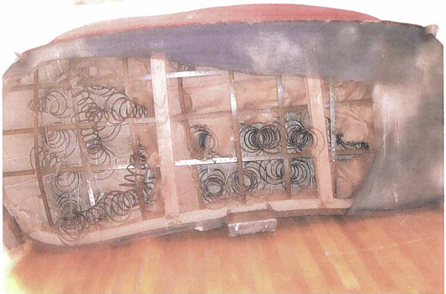
Bottom of couch was soaked, causing old Fashioned spring ties to break and bottom berlap cover to give way
