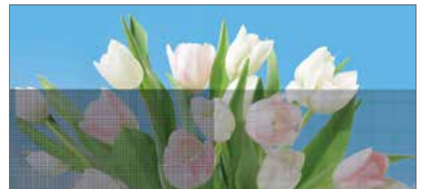
View through regular fiberglass insect screen
