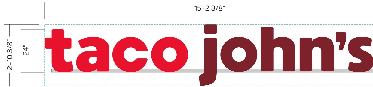
CHANNEL LETTER DETAIL SCALE: 3/8" = 1'-0"
