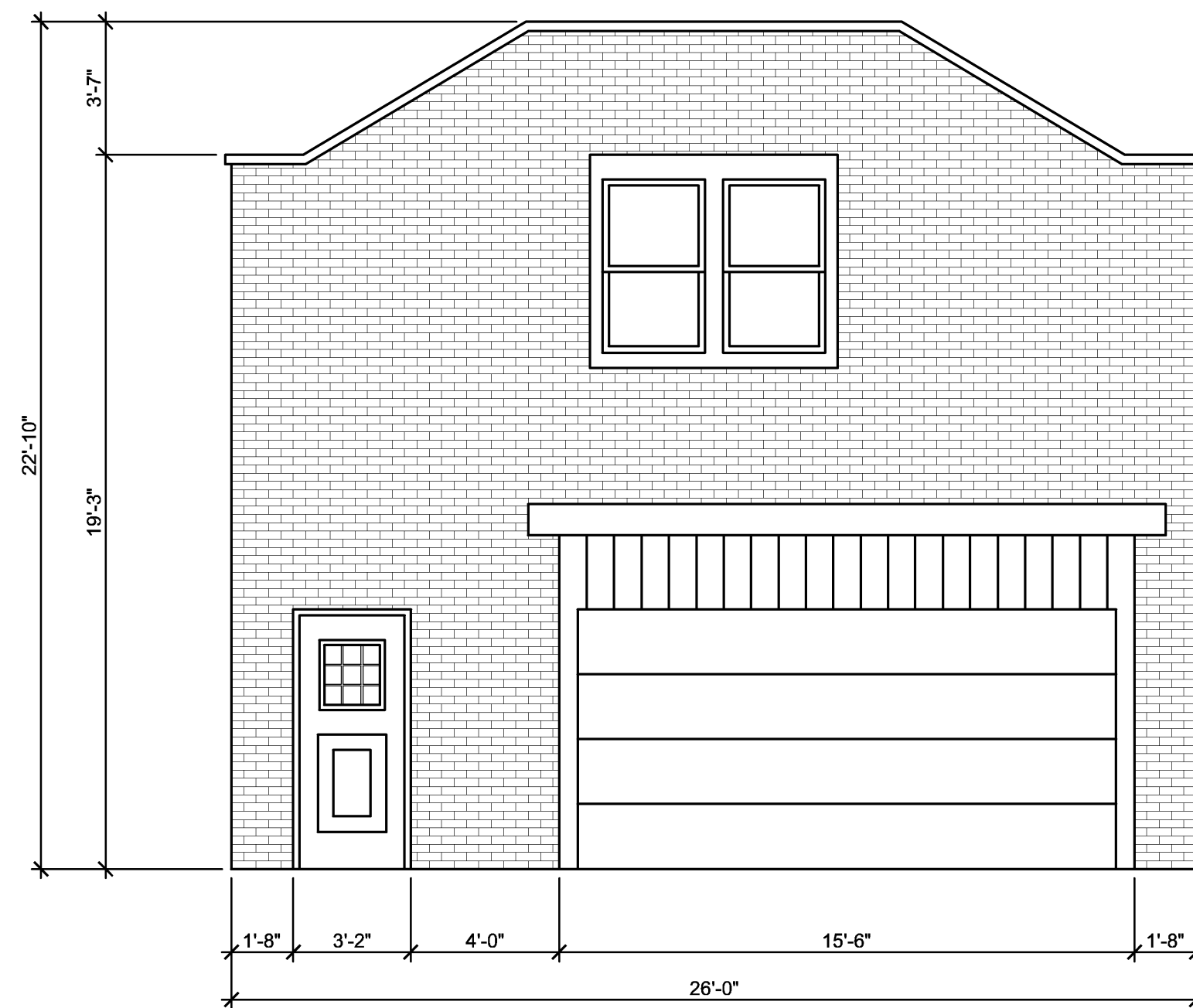
COACH HOUSE EXISTING NORTH ELEVATION 1/4" = 1'-0"
