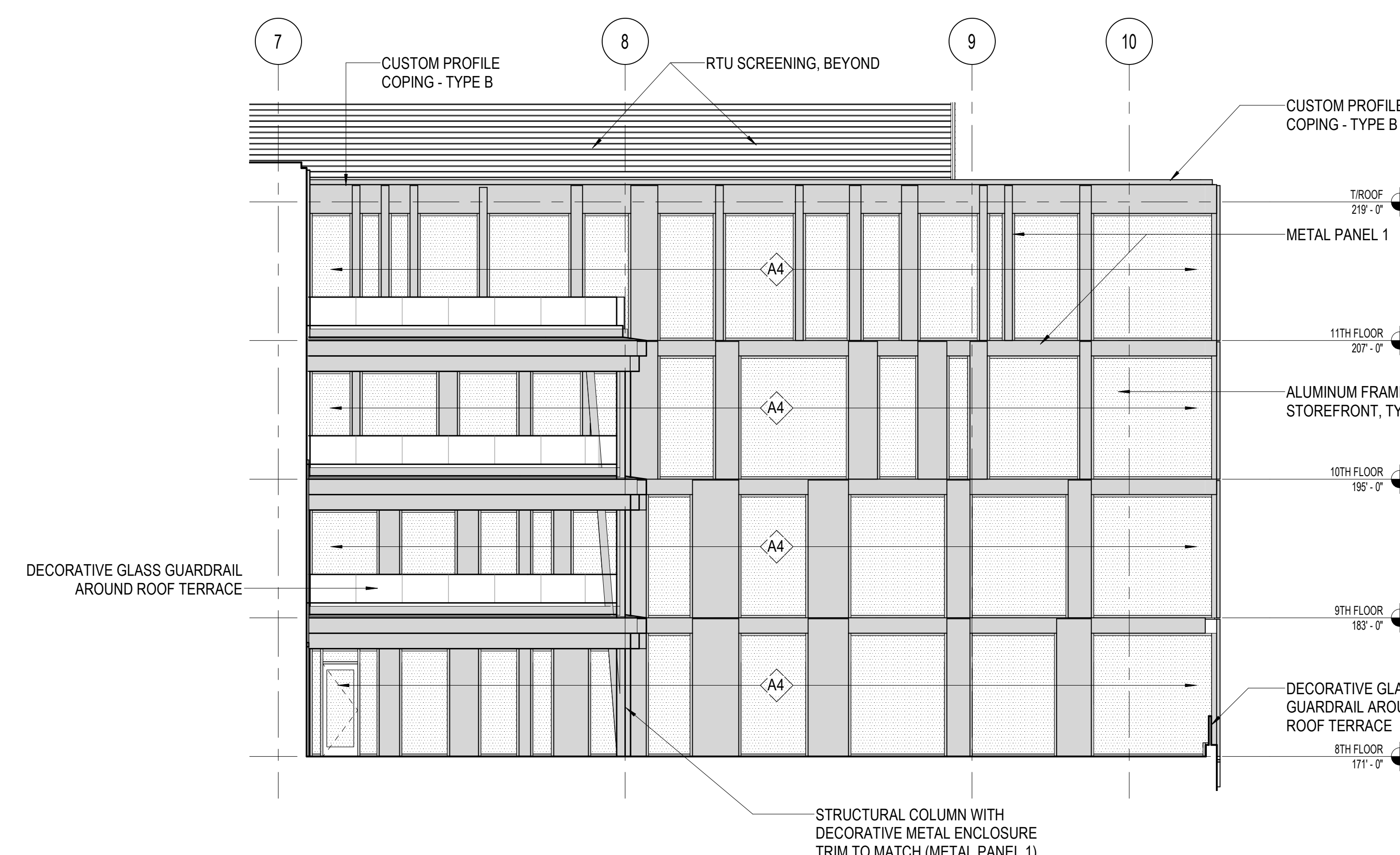
3 PARTIAL EAST ELEVATION - TERRACE SCALE: 1/8" = 1'-0"
