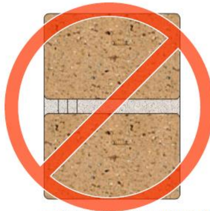
7. FINAL PASS INCORRECTLY SMEARED ABOUT BRICK EDGES RESULTS IN EXAGGERATED JOINT WIDTH
