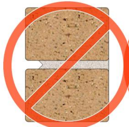
2. JOINT GROUND TO INCORRECT PROFILE
