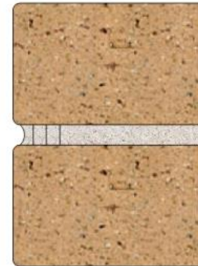
8. FINAL PASS TOOLED TO CONCAVE OR VEE PROFILE TO MATCH EXISTING
