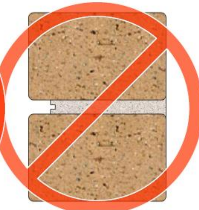
3. JOINT GROUND TO INCORRECT PROFILE
