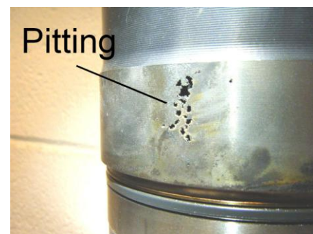
Cylinder liner, due to lack of coolant
