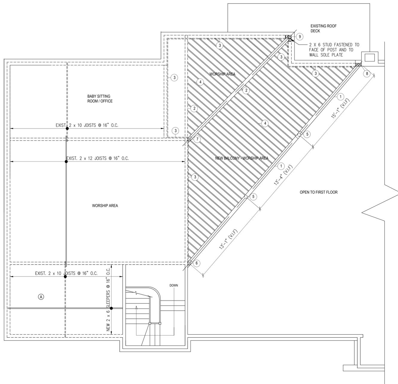
1 SECOND FLOOR FRAMING PLAN (FLOOR DECKING NOT SHOWN FOR CLARITY)
