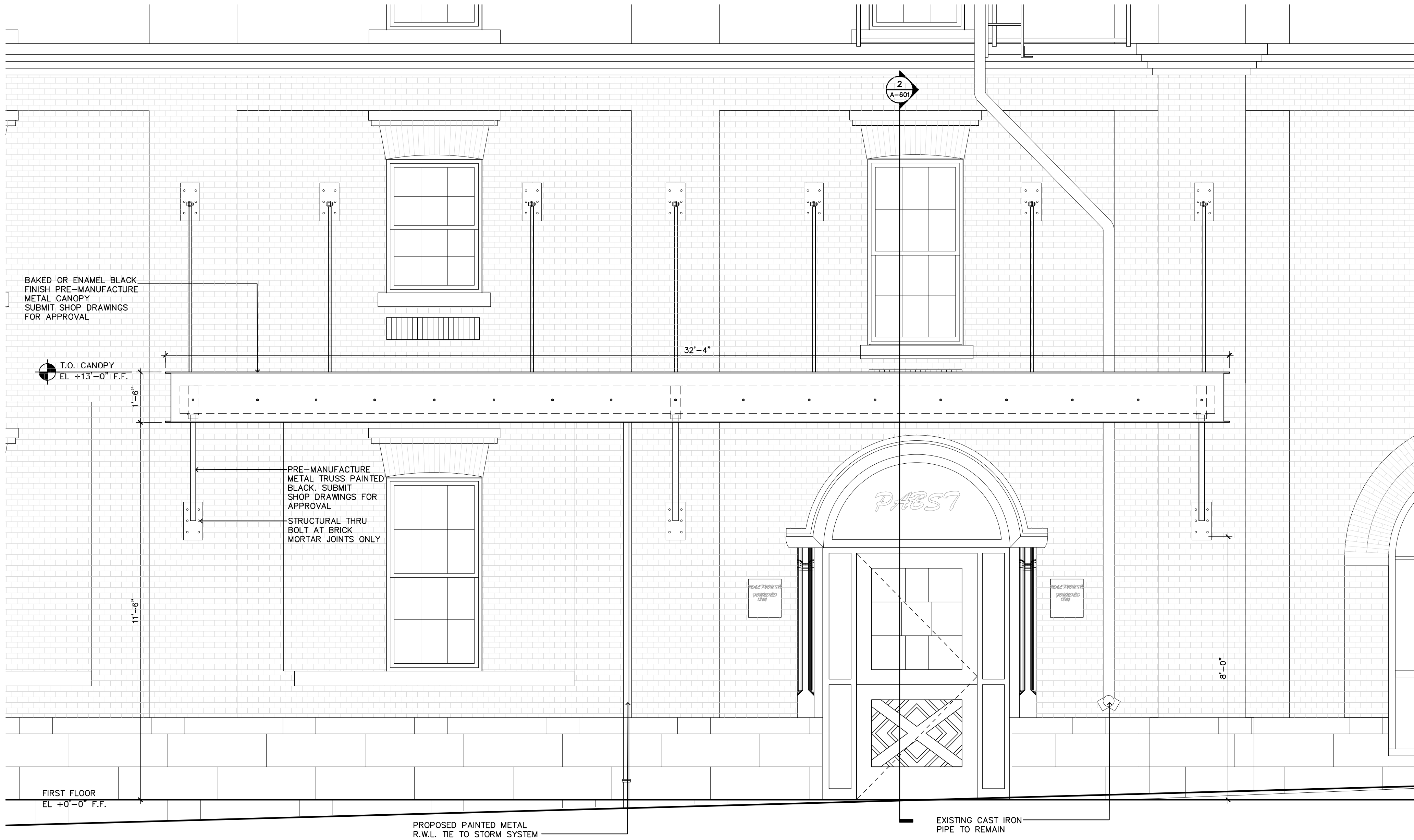
1 PARTIAL BUILDING ELEVATION PROPOSED ENTRANCE CANOPY SCALE: 1/2" = 1'-0"
