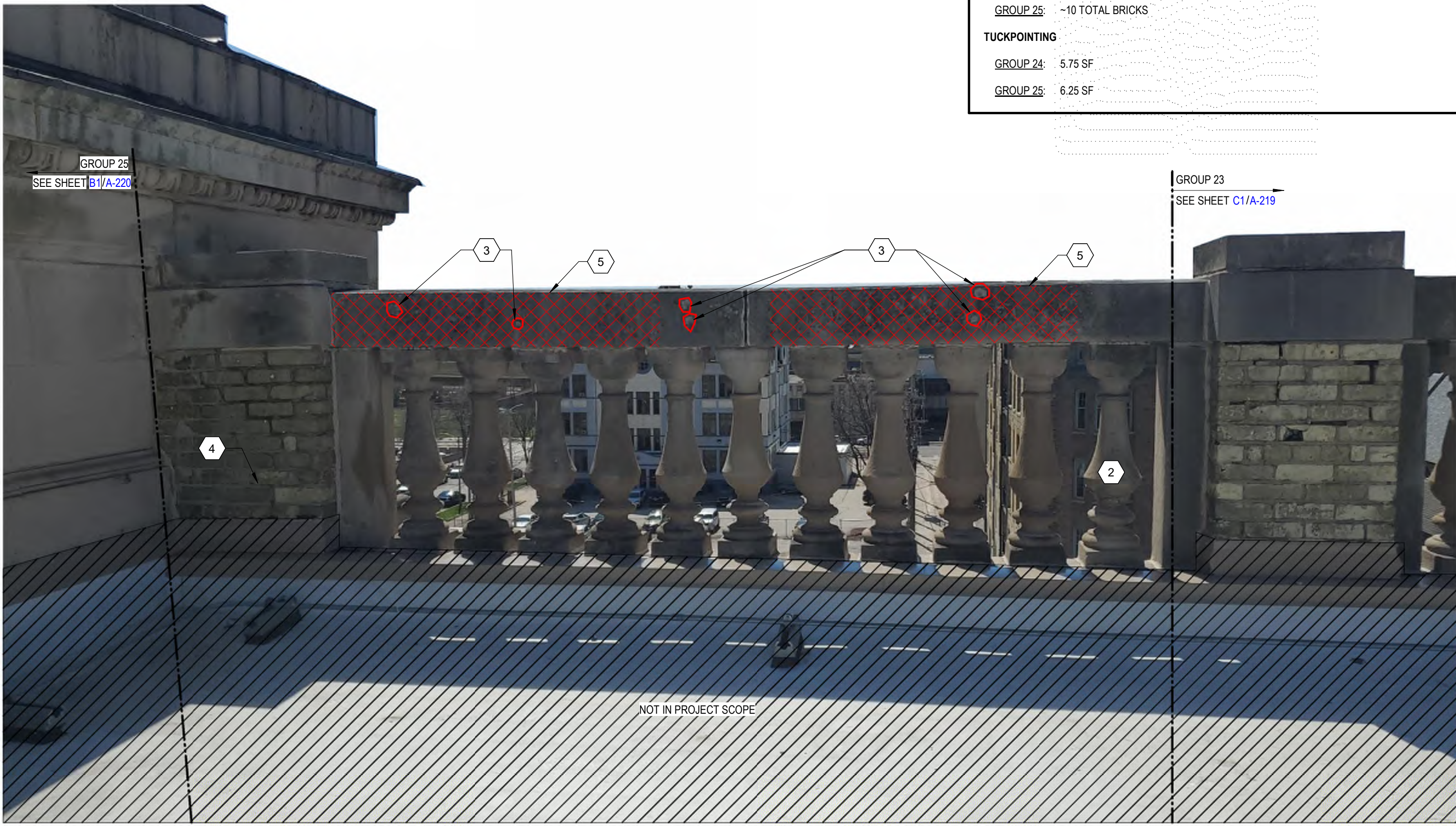
C4 GROUP 24 - SOUTH - INTERIOR ELEVATION OF SPINDLES
