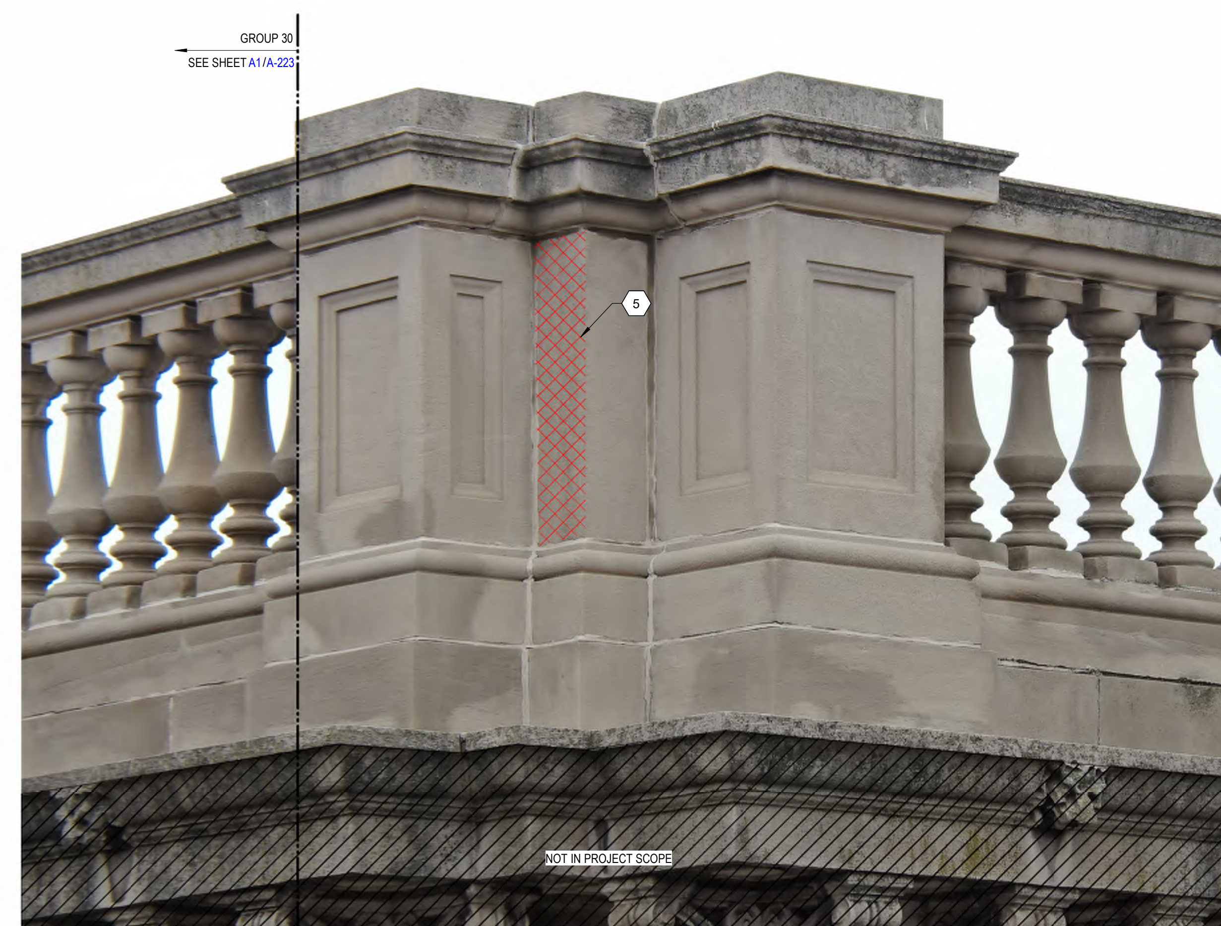
A4 GROUP 31 - SOUTH - EXTERIOR ELEVATION OF SPINDLES
