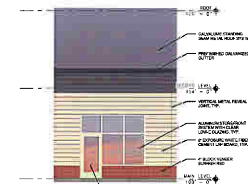
6 PARTIAL MULTI-SPACE SOUTH ELEVATION 3/16" = 1'-0"
