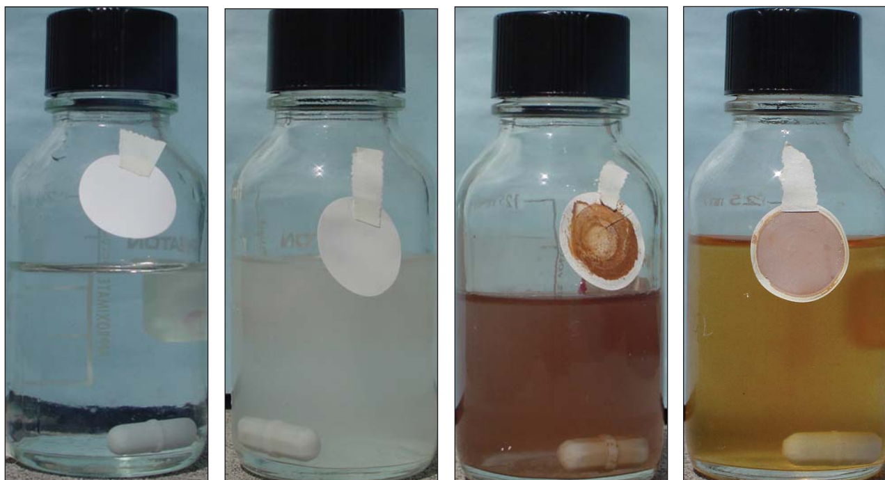
At pH 5.5, solutions with 48,000 µg/L Pb +2 are clear because most of the lead is soluble (far left). At pH 8.5, a white solid precipitates (middle left). When chlorine is present at pH 5.5 or 8.5, a highly insoluble red-brown solid precipitates (middle right). The red-brown solids are hard to distinguish from “red water” samples caused by corroding iron (far right). The filter paper attached to each container indicates the color of the captured particles.
