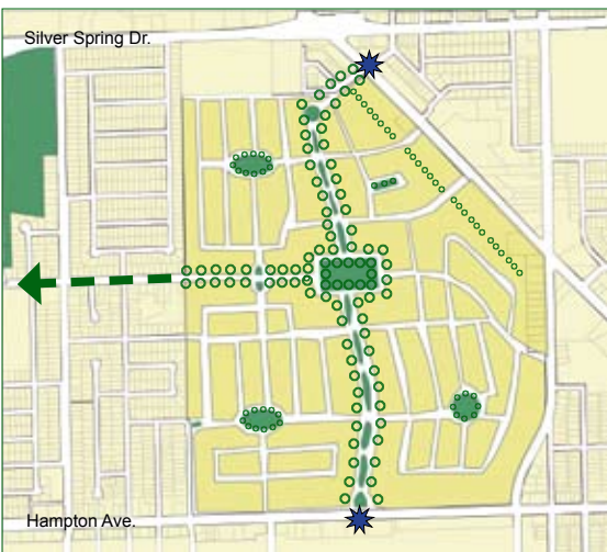
This sketch diagram illustrates one possible street and block layout for a 'Traditional Neighborhood Design' in the Timmerman Airport area (see Dist 8 Recommendations 4:16-4:17). Key concepts include a connected street grid, street layout that deters 'cut through' traffic, multiple and connected greenspaces, entrance gateways, and limited commercial lots along major arterials.
