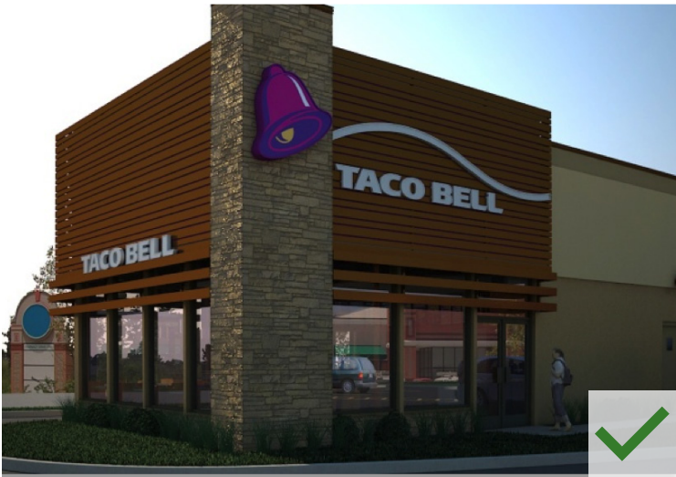
MAIN SIGNAGE COMPONENTS (i.e., wave form element, letterset, bell) should occupy centerline of slat wall and letterset should be at horizontal center line of bell logo
