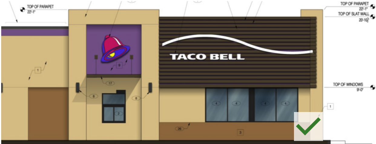
WAVE FORM ELEMENT AND LETTERSET LAYOUT centered on horizontal centerline of bell logo.
