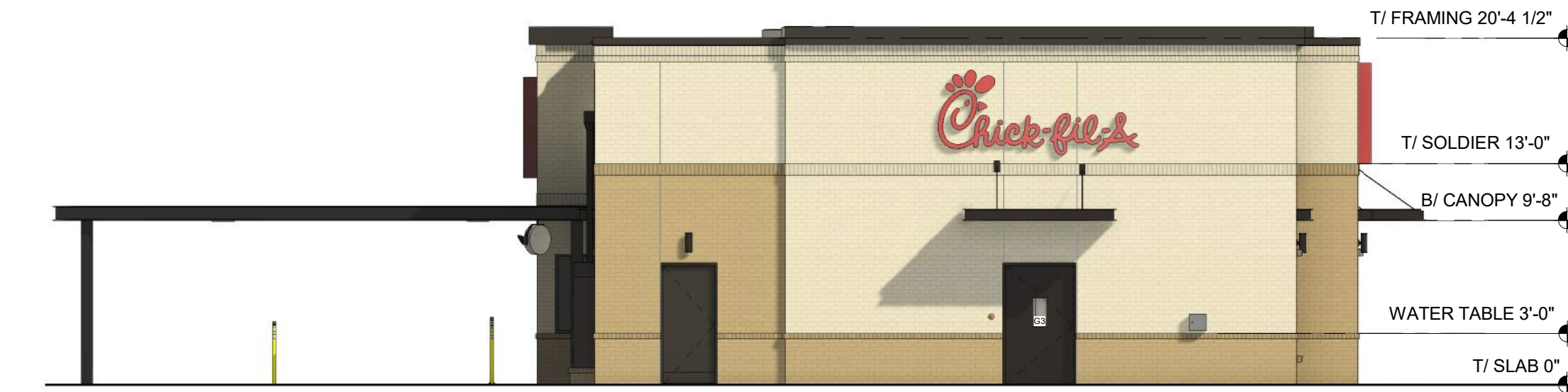
4 WEST EXTERIOR ELEVATION 1/8" = 1'-0"
