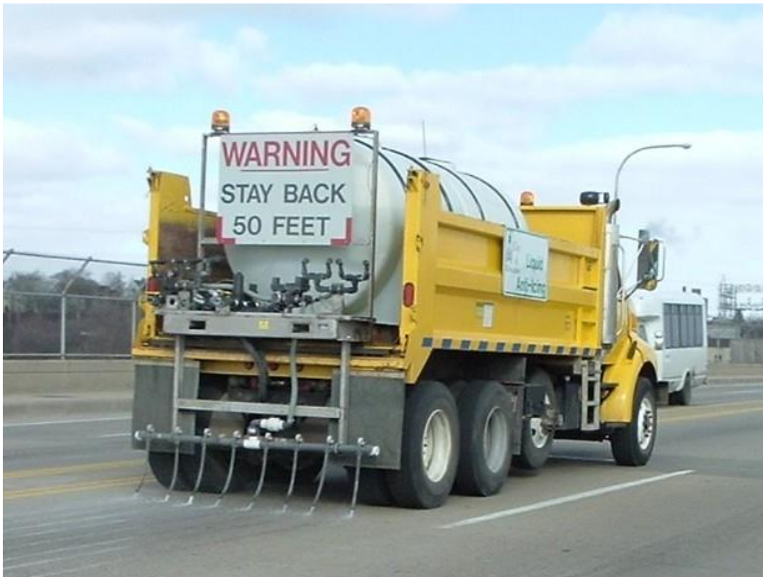
DPW truck applying brine to the pavement over a viaduct
