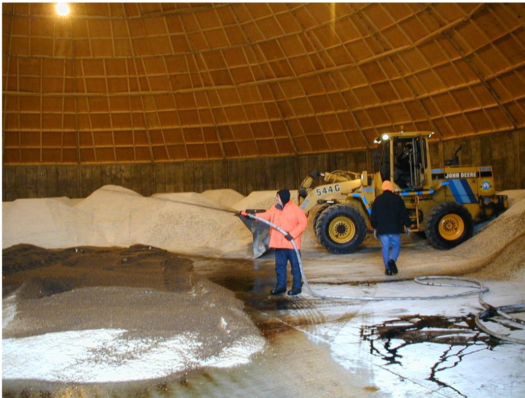
City staff spraying GEOMELT® onto rock salt
