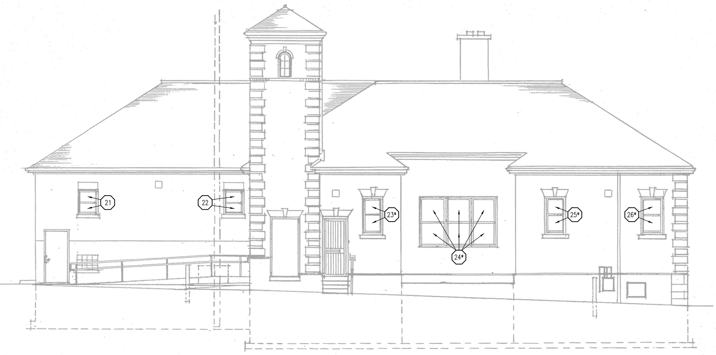
D4 A400 WEST EXTERIOR ELEVATION GLAZING REPLACEMENT 1/8" = 1'-0"
