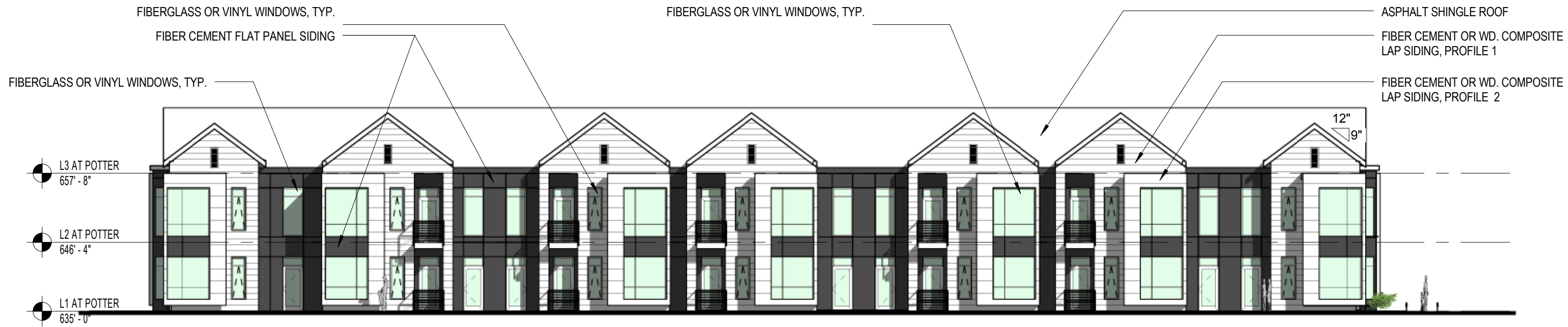
BUILDING A - SOUTH ELEVATION
