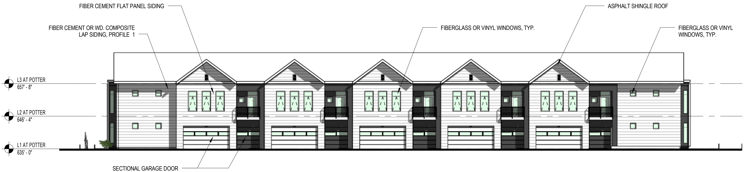
BUILDING A - NORTH ELEVATION
