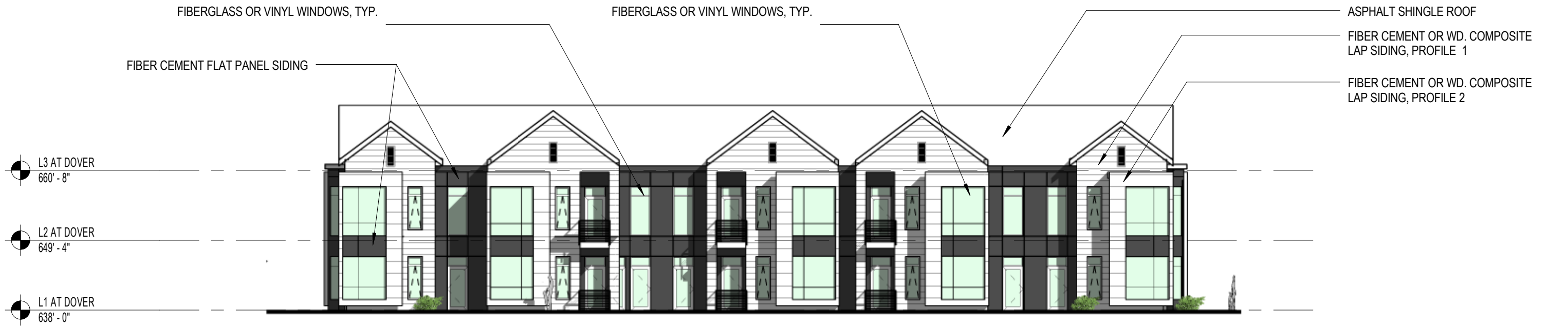
BUILDING B - NORTH ELEVATION
