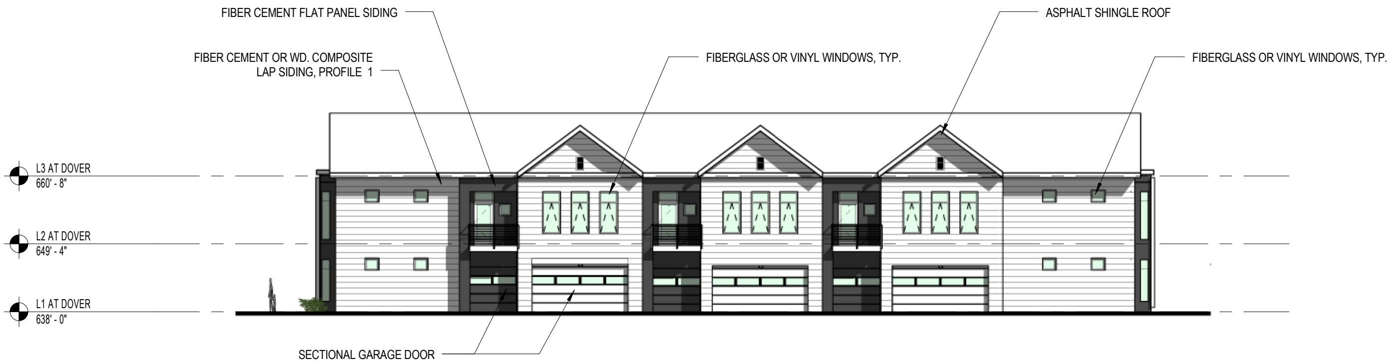
BUILDING B - SOUTH ELEVATION
