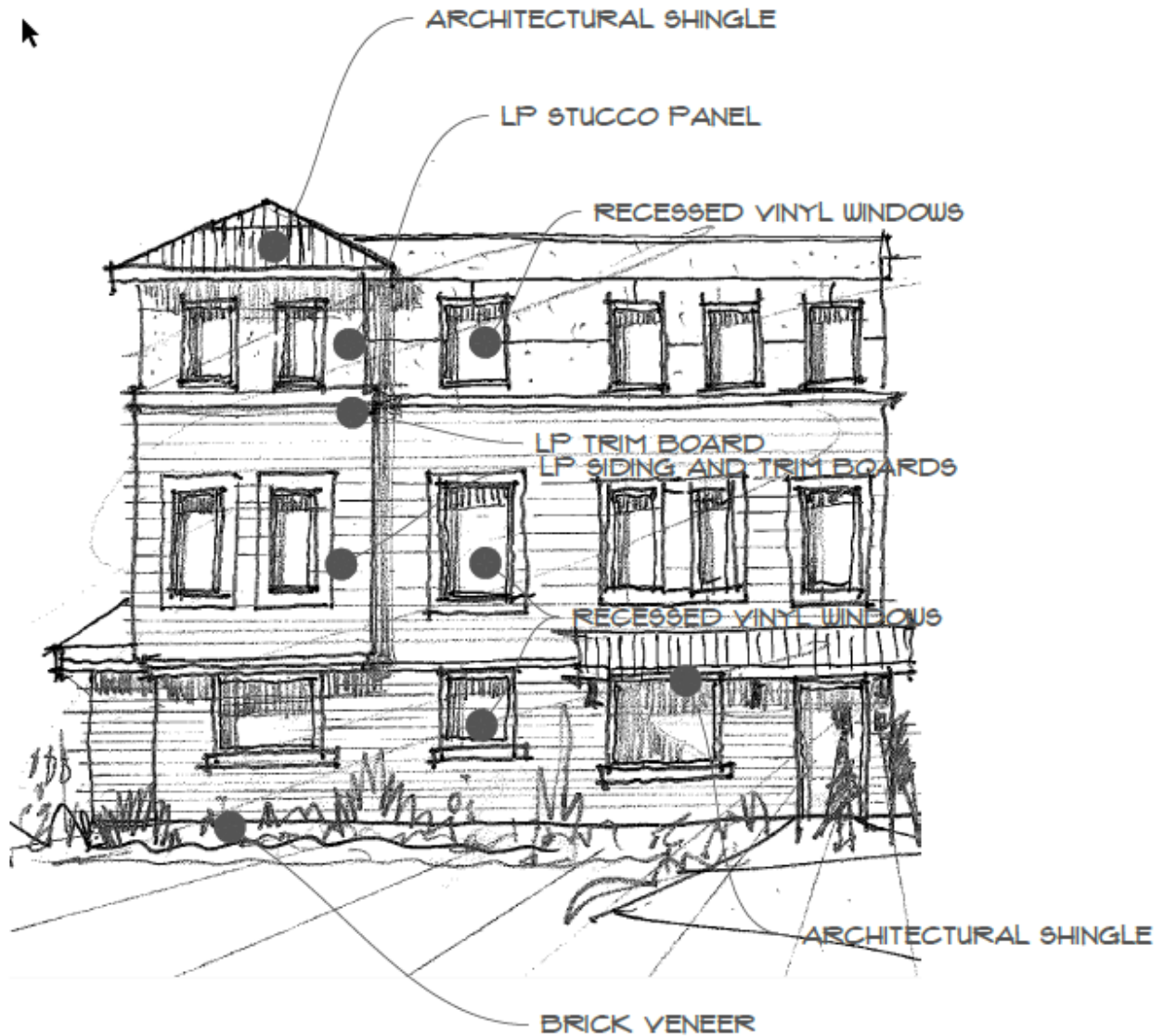
PARTIAL ELEVATION STUDY WITH TYPICAL EXTERIOR FINISHES
