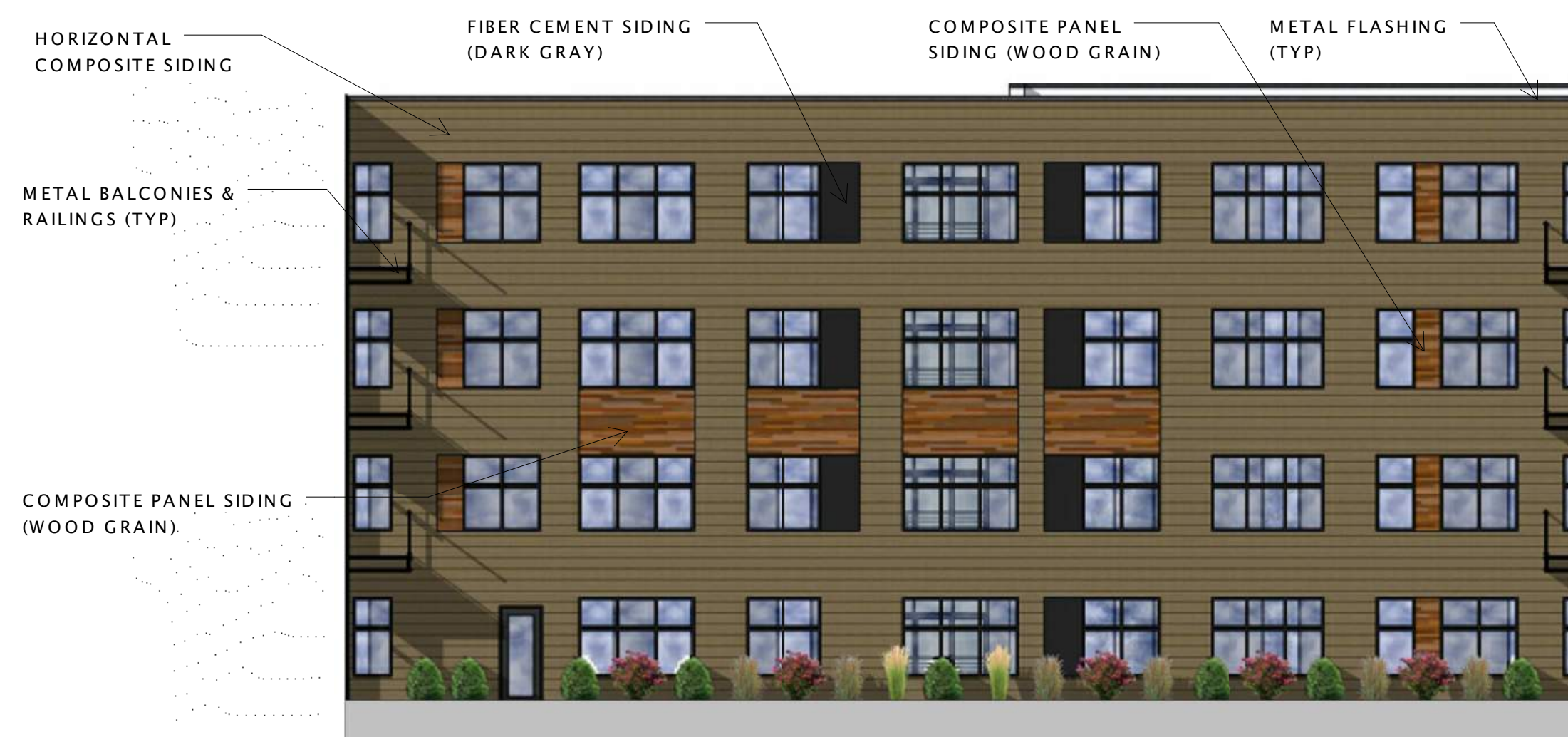
8 Courtyard West Elevation 3/32" = 1'-0"
