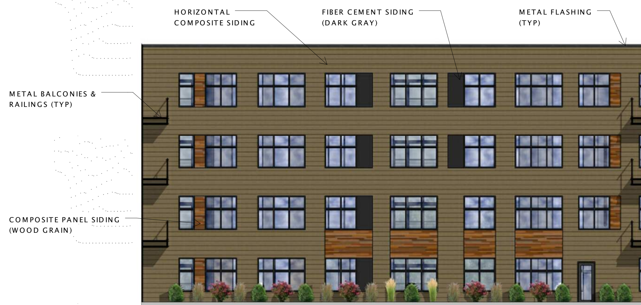
18 Courtyard East Elevation 3/32" = 1'-0"
