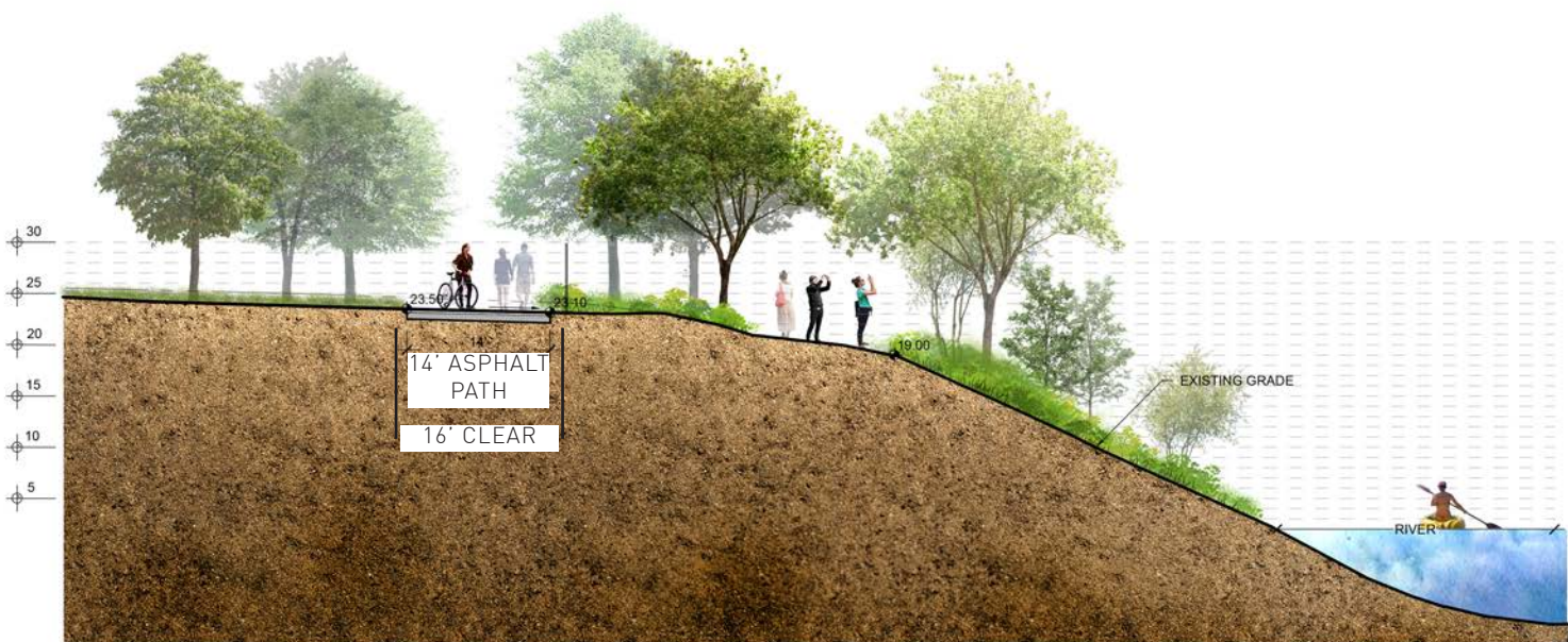
PROPOSED GRADING CONDITION SECTION
