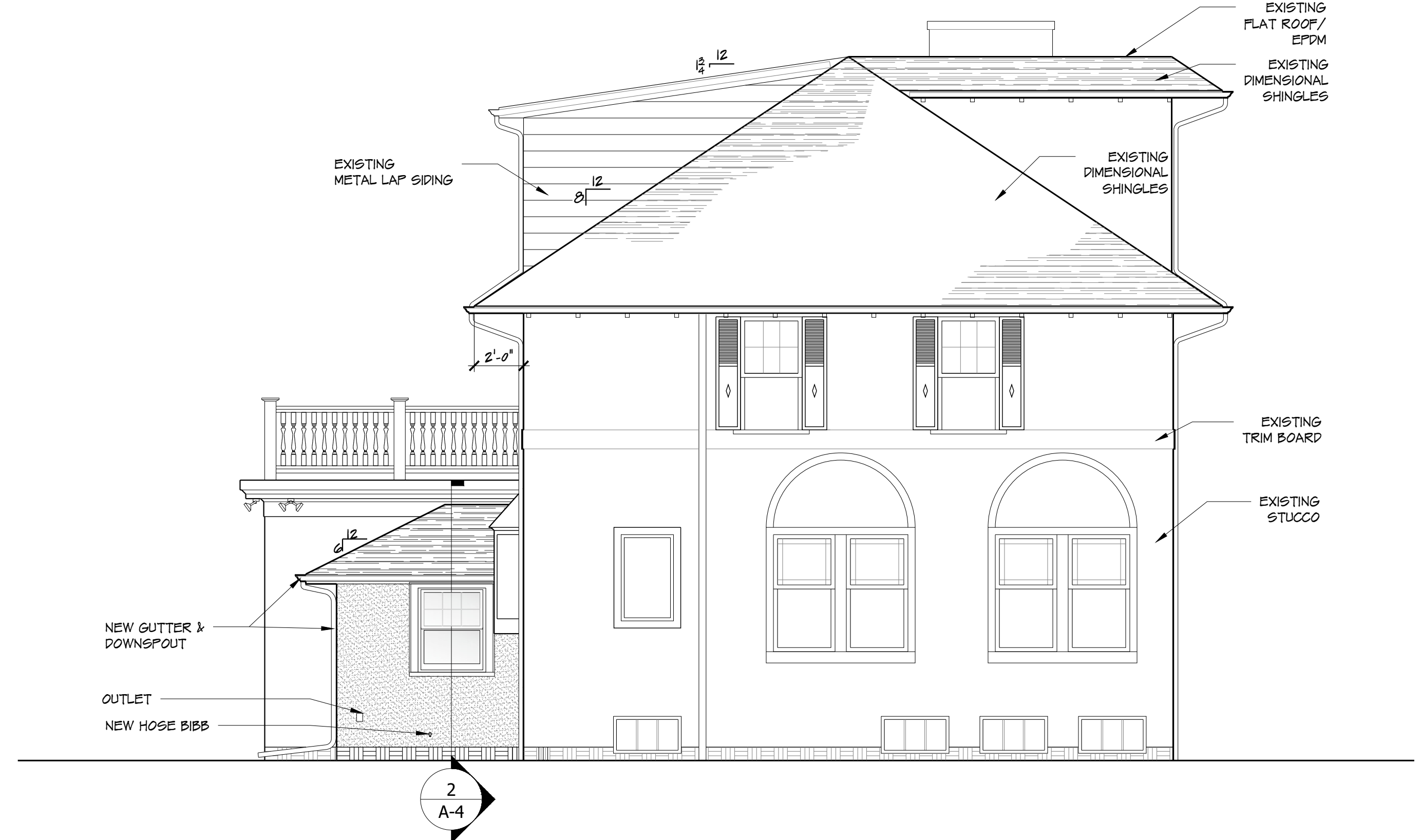
PROPOSED NORTH ELEVATION 1/4" = 1' - 0"
