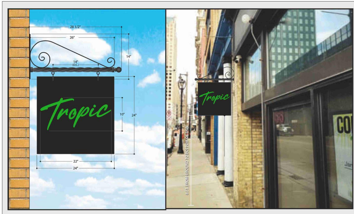
24" w x 24" h size double sided non-illuminated aluminum hanging panel sign Logo to be 1/4" raised acrylic with green vinyl face (quantity 1)
