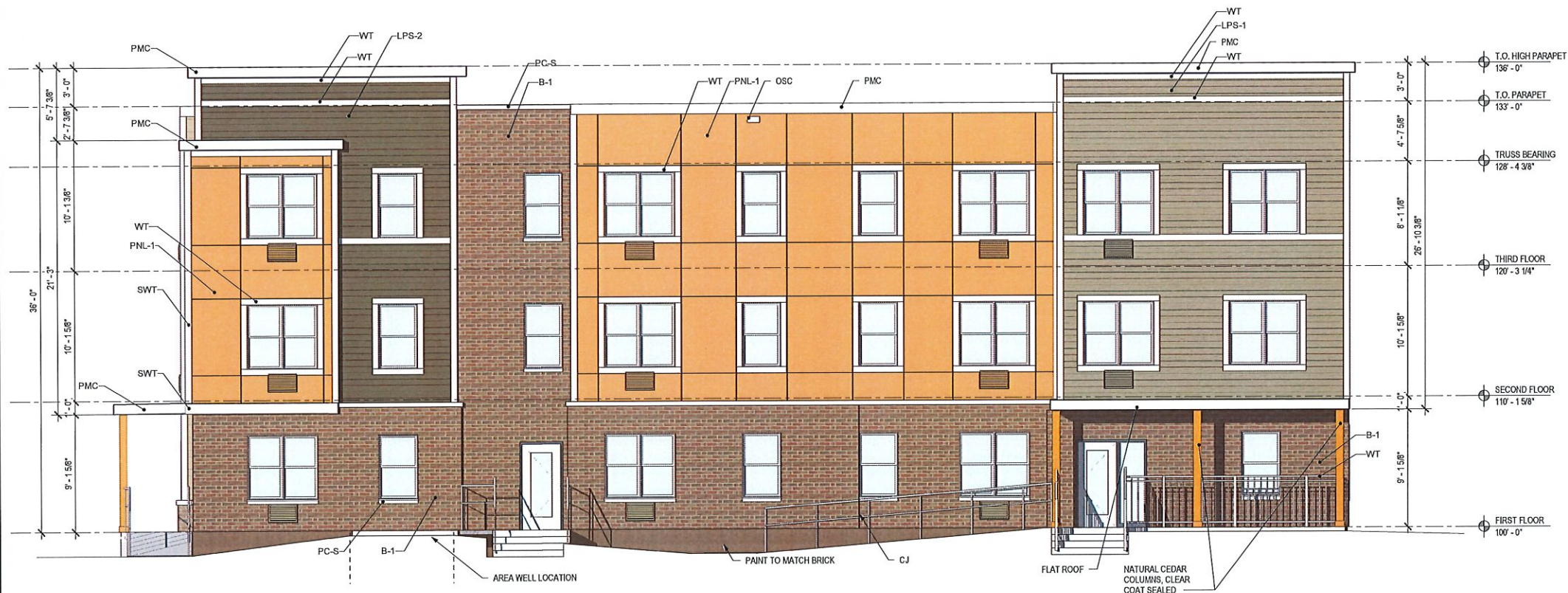
1 EXTERIOR ELEVATION - SOUTH 3/16" = 1'-0"
