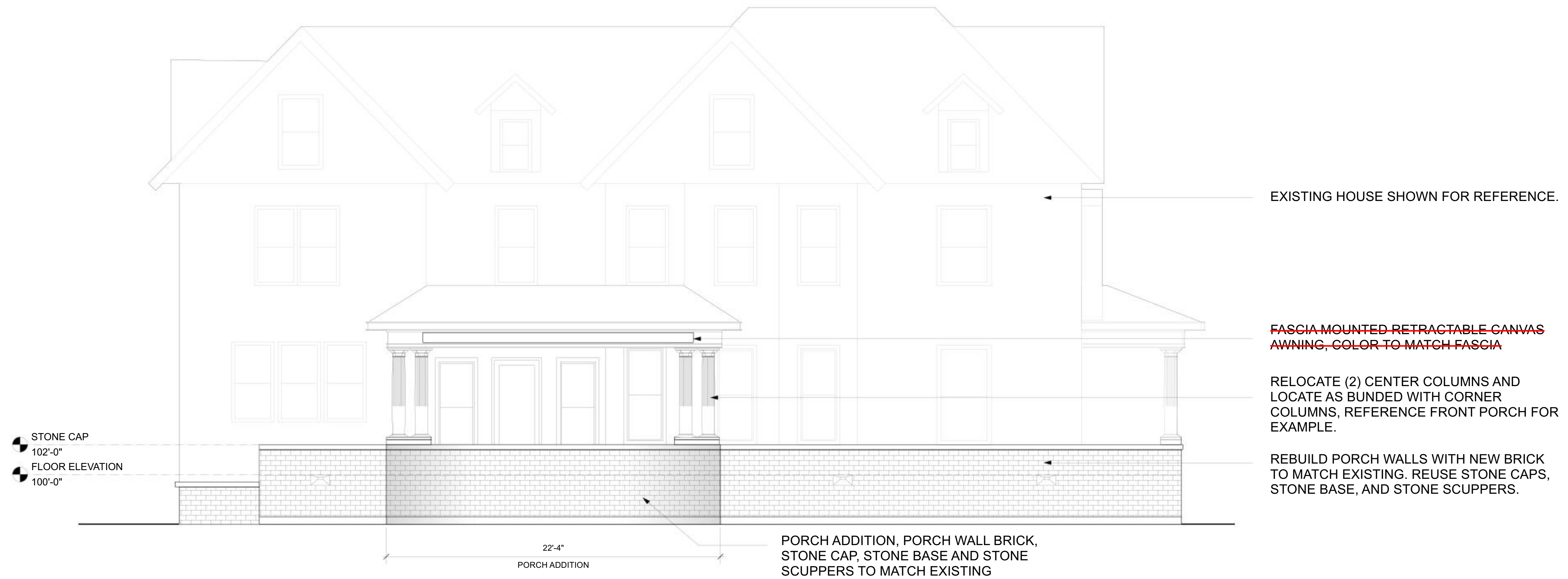
1 SOUTH WEST ELEVATION OF PORCH Scale: 1/4" = 1'-0"
