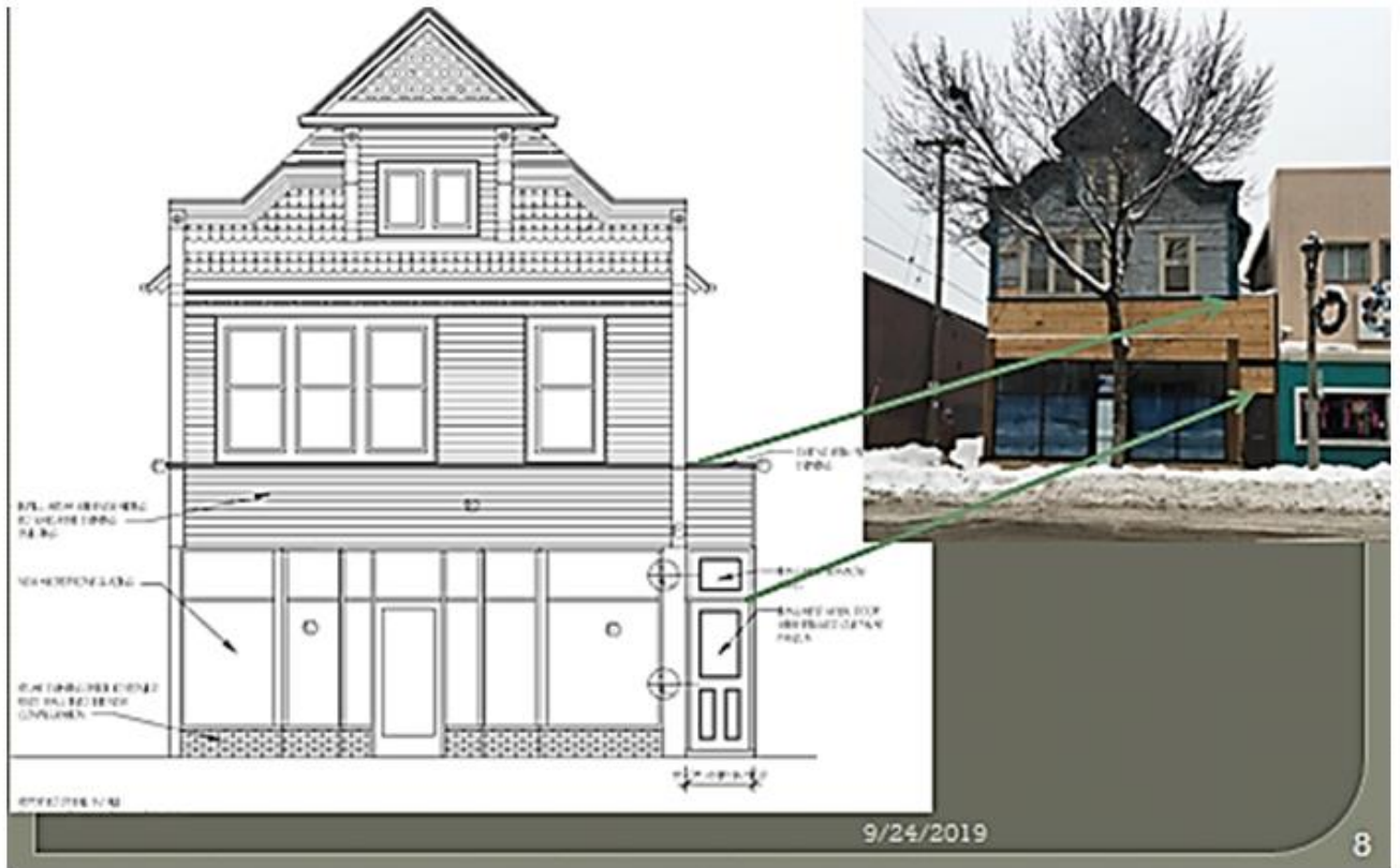
Approved elevation at left with inset photo showing departure from plans
