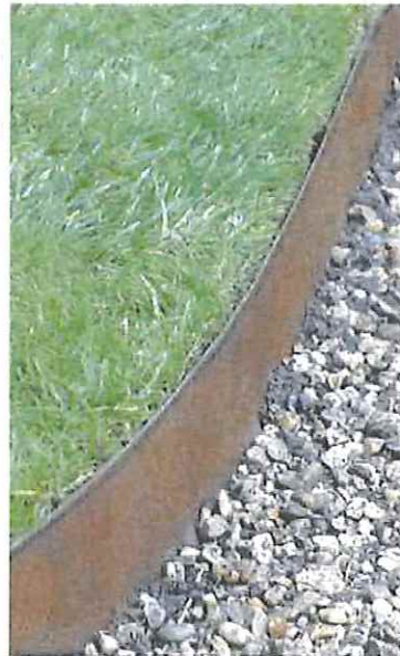
CorTen steel edging around all perennial beds. Minimum 14 Gauge thickness. 8" above finished grade errand perennials. 3" above grade between lawns and compacted limestone areas. Provide samples of all materials prior to construction.
