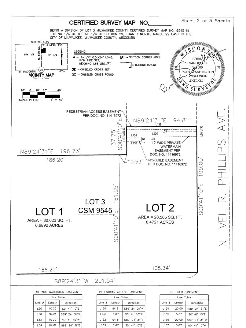
HORIZONTAL DATUM IS THE WISCONSIN STATE PLANE COORDINATE SYSTEM SOUTH ZONE NAD27. NORTH IS REFERENCED TO THE W. LINE OF THE NE 1/4 OF SECTION 29-7-22 PUBLISHED BY SEWRPC AS NO0'54'02"E. ALL DISTANCES ARE GROUND MEASURED. (DEC. 2013 DATUM)
