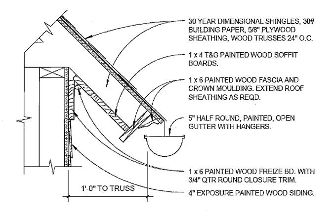
3 TYPICAL EAVE - GABLE SIMILAR 1 1/2" = 1'-0" A BOXED SOFFIT WILL NOT BE CONSTRUCTED AND THE PLATE ROOF SHOWN HERE WILL BE CONSTRUCTED
