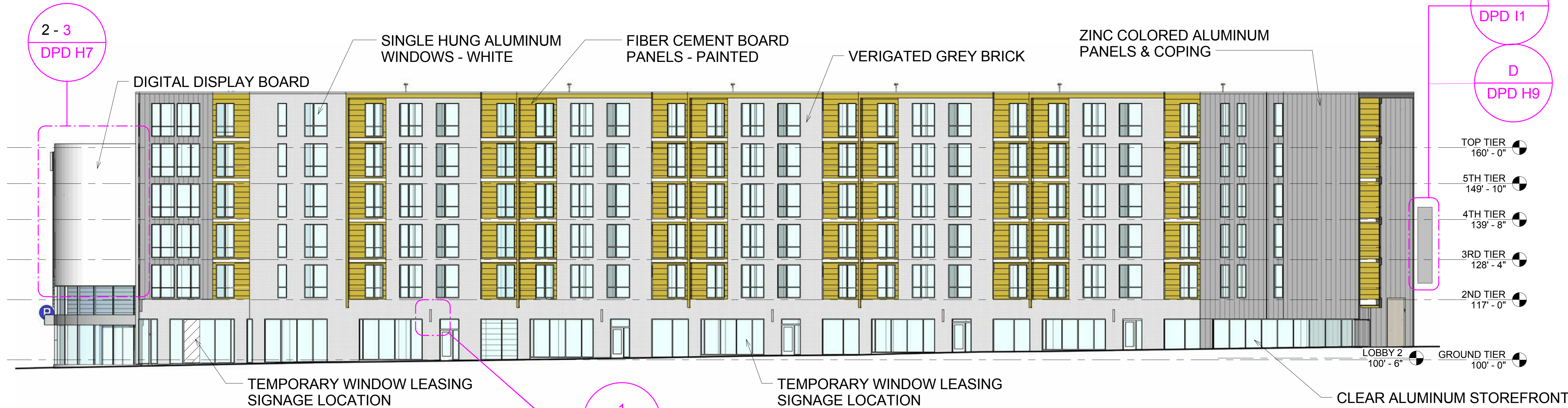
5 WEST ELEVATION WITH HOUSING (DPD)
