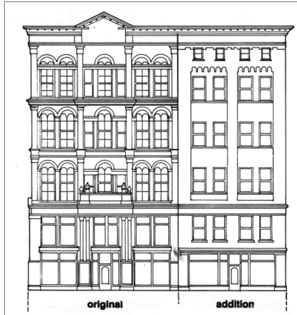
Sensitive Addition: Iron Block Building, Milwaukee, Wisconsin
