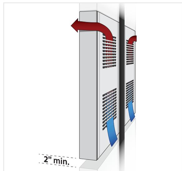
**DO NOT RESTRICT AIRFLOW** on the cabinet's rear side. A minimum 2" gap per face behind each cabinet is necessary. For wall-mounted rear-vent cabinets, airflow must be unobstructed from top to bottom, in addition to leaving a minimum 3" gap between the sign and wall.
