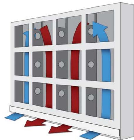
**DO NOT BLOCK** the air intake, exhaust or LED modules located on the front face with any part of the metal cabinet or coverings.
