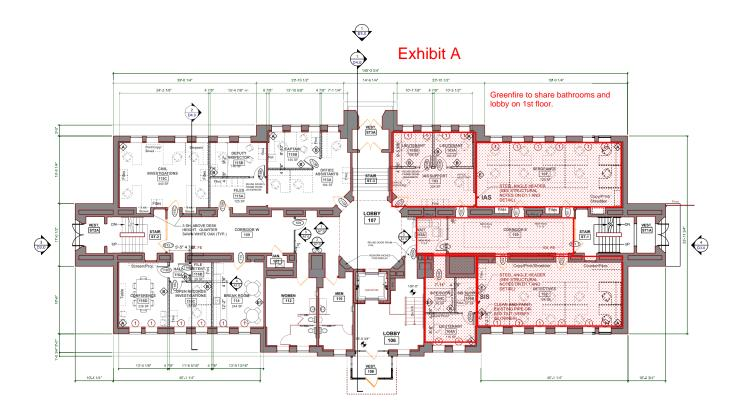
EX. FE - EXISTING FIRE EXTINGUISHER CURRENT MEETS CODE 75" TRAVEL DISTANCE, VERIFY WITH BUILDING INSPECTOR IF ADDITIONAL IS REQUESTED. ANY ADDITIONAL FE TO BE SEMI-RECESSED
