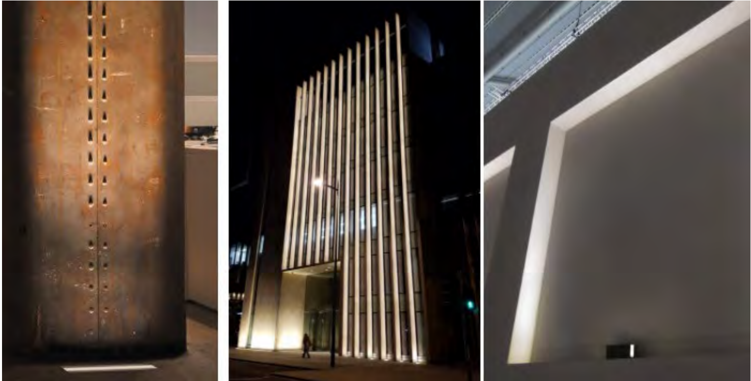
Lighting example for vertical reveal
