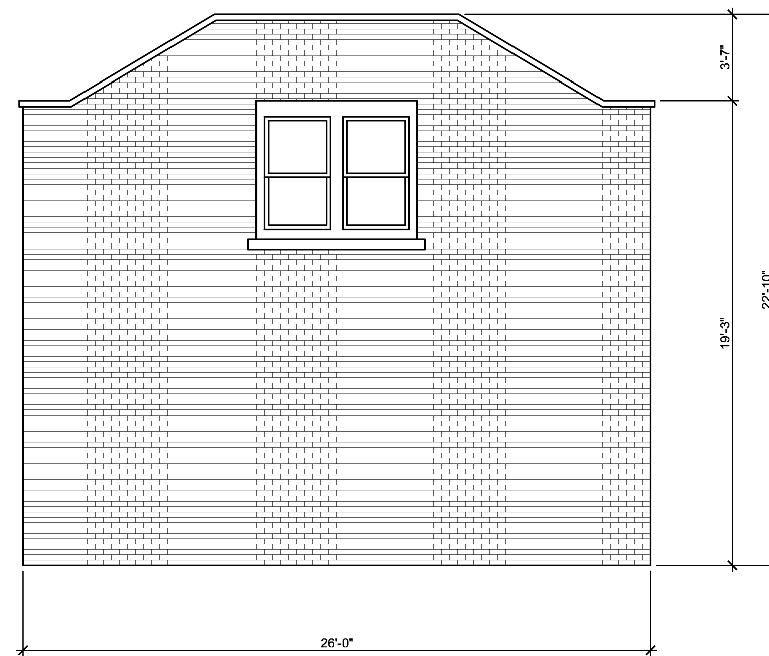
COACH HOUSE EXISTING SOUTH ELEVATION 1/4" = 1'-0"
