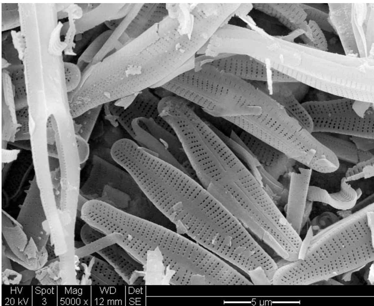
Figure C.69 SEM image of bottom of meter #1. The particles are skeletons of diatoms that have been incorporated in the scale.
