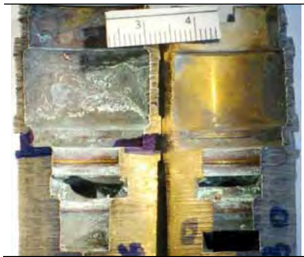
Figure F.127 Macro photograph of Interior Surfaces of Faucets at Site F1 (left) and F2 (right)
