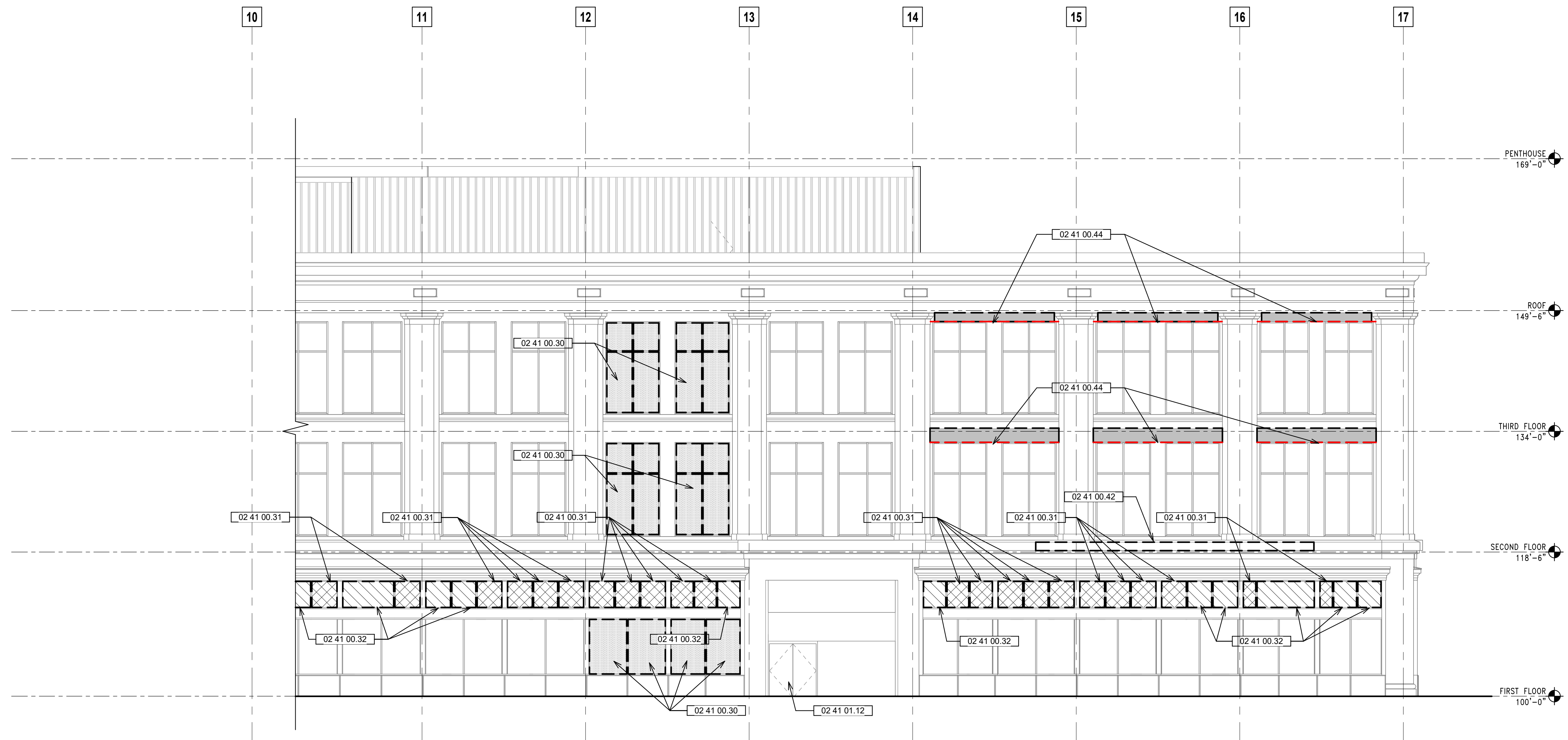
2 SOUTH ELEVATION - EAST END - DEMOLITION SCALE: 1/8" = 1'-0"
