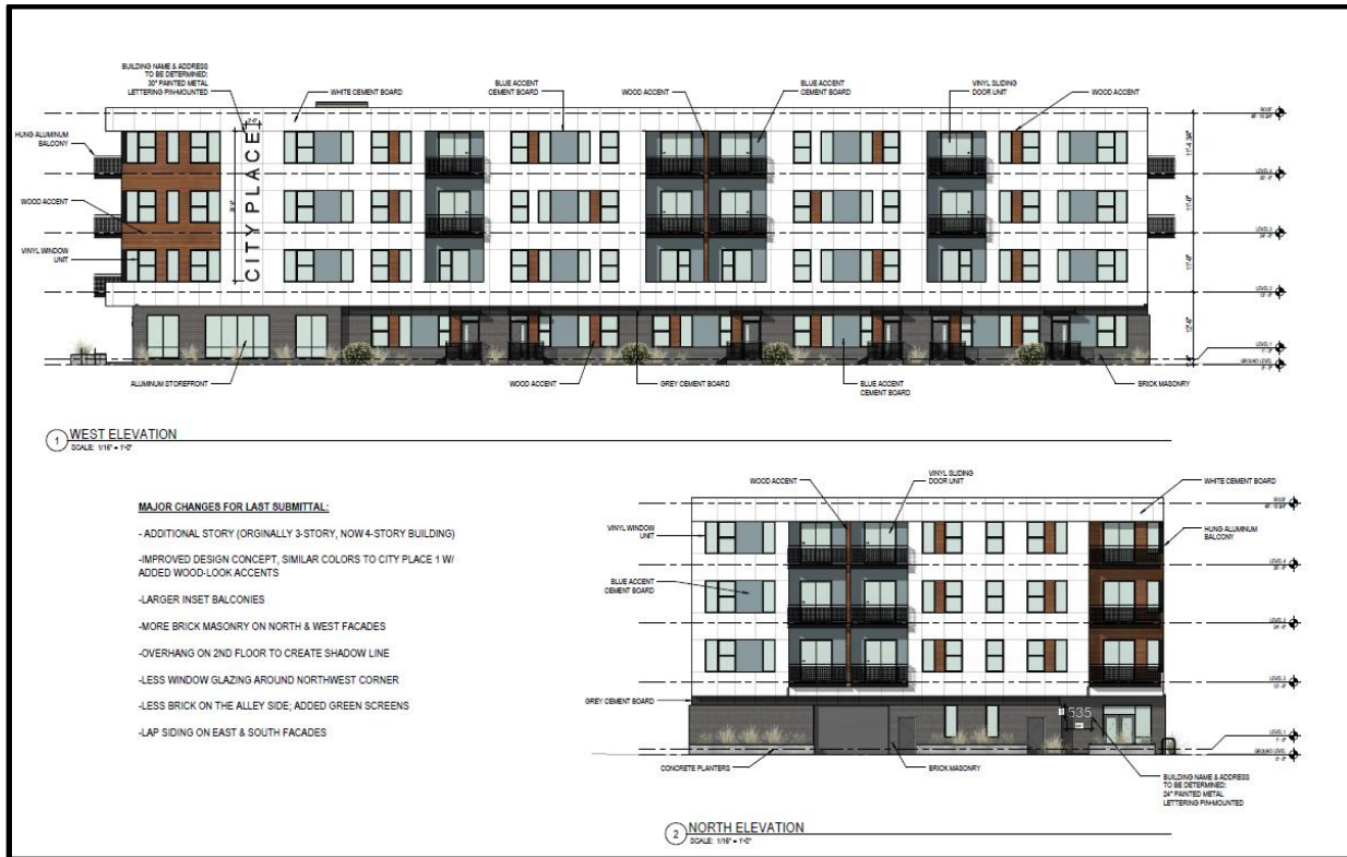
1728 North 6th Street Elevations
