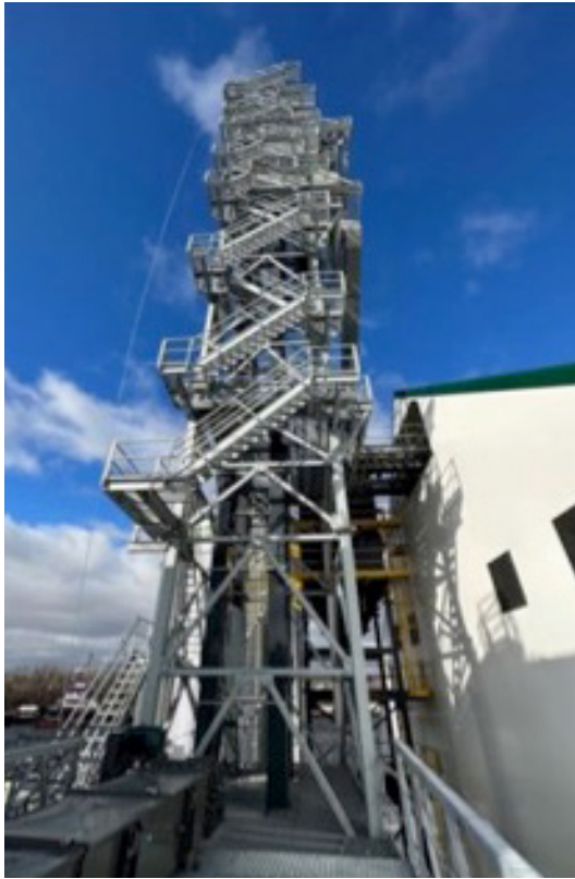
Figure 10: Bucket Elevator and Distributor
