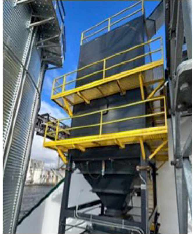
Figure 11: Bulk Scale for Load-Out
