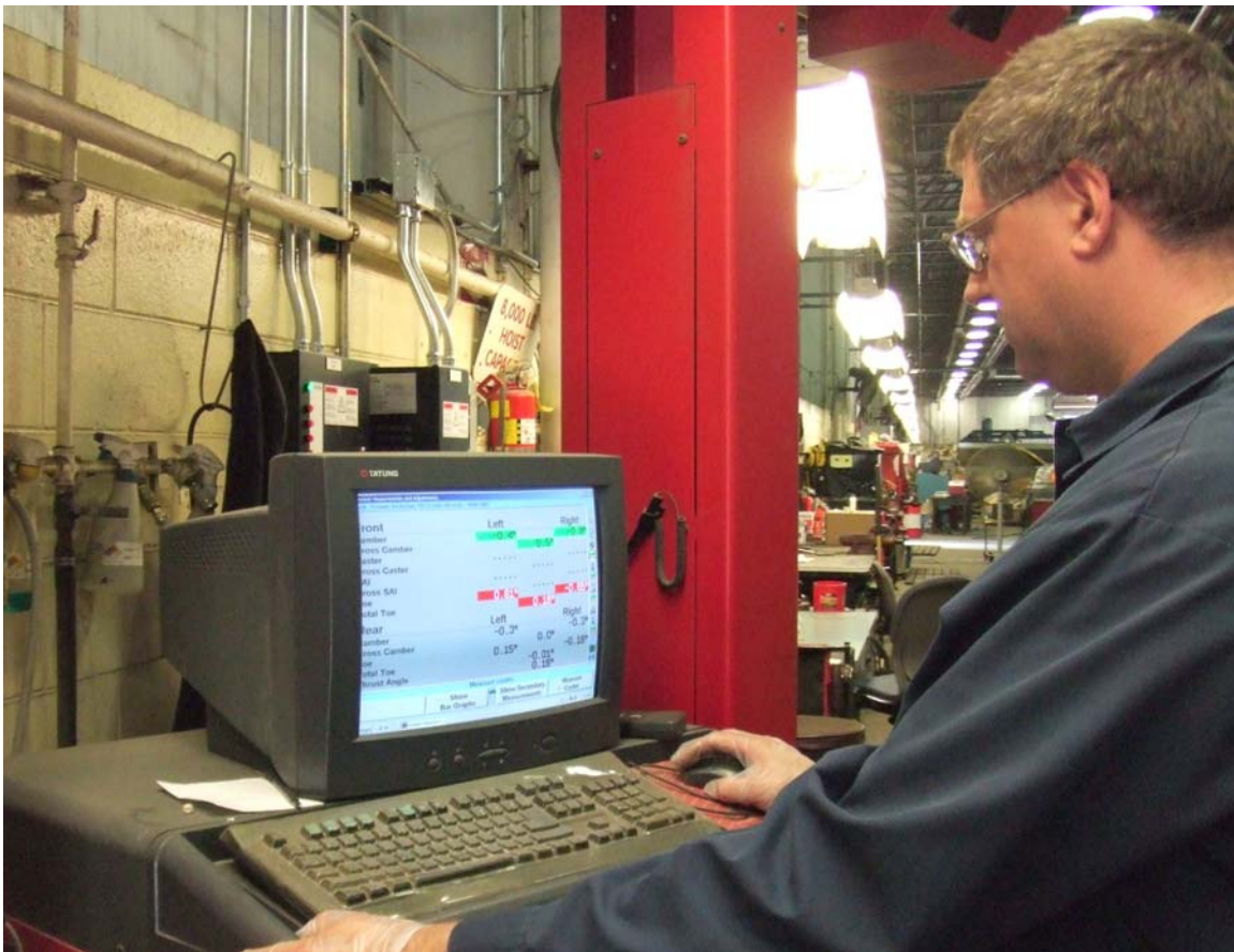
James Kehoss performing an alignment on the new computerized front end alignment machine. This unit has the capability to perform both 2 and 4 wheel alignments.
