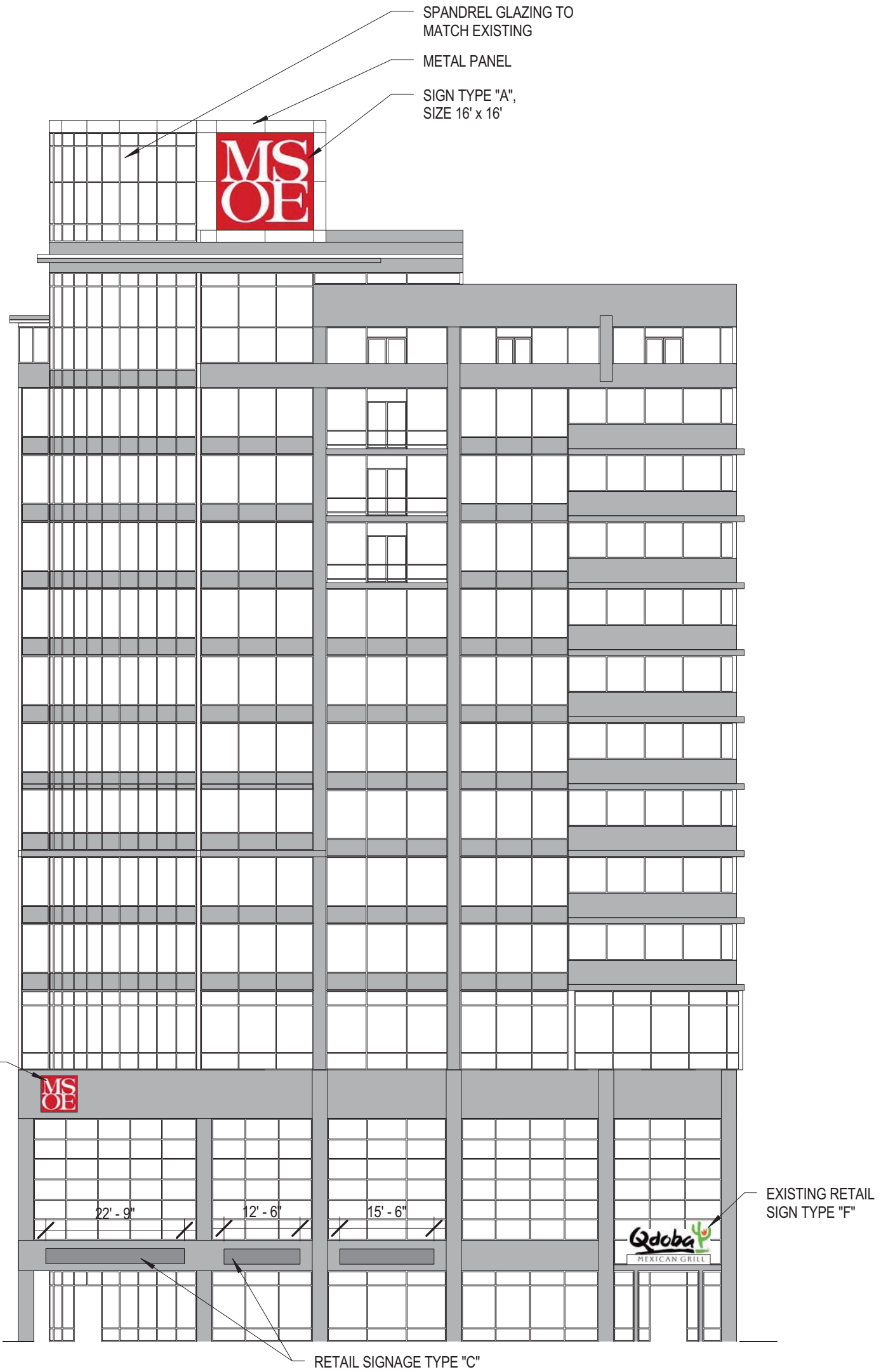
1 WEST EXTERIOR ELEVATION 1" = 20'-0"
