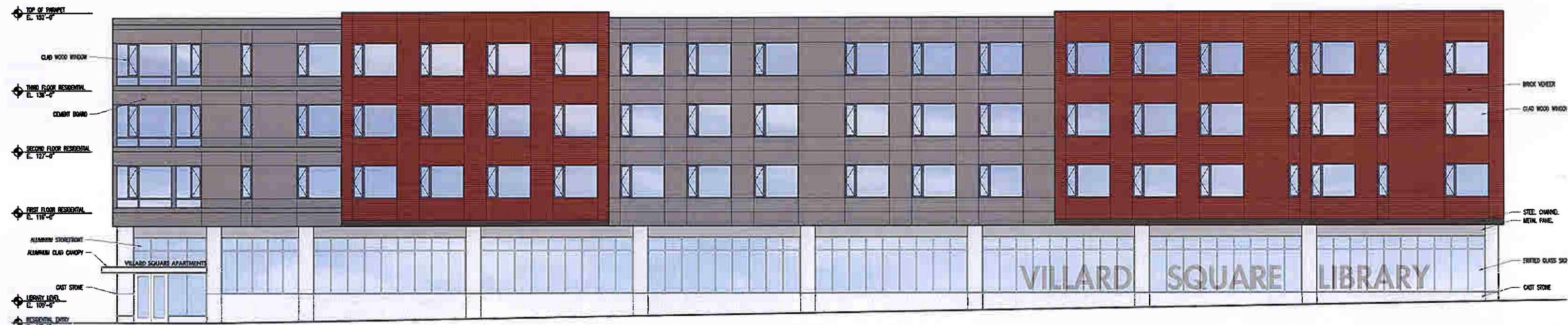
WEST VILLARD AVENUE ELEVATION SCALE: 1/8"=1'-0"
