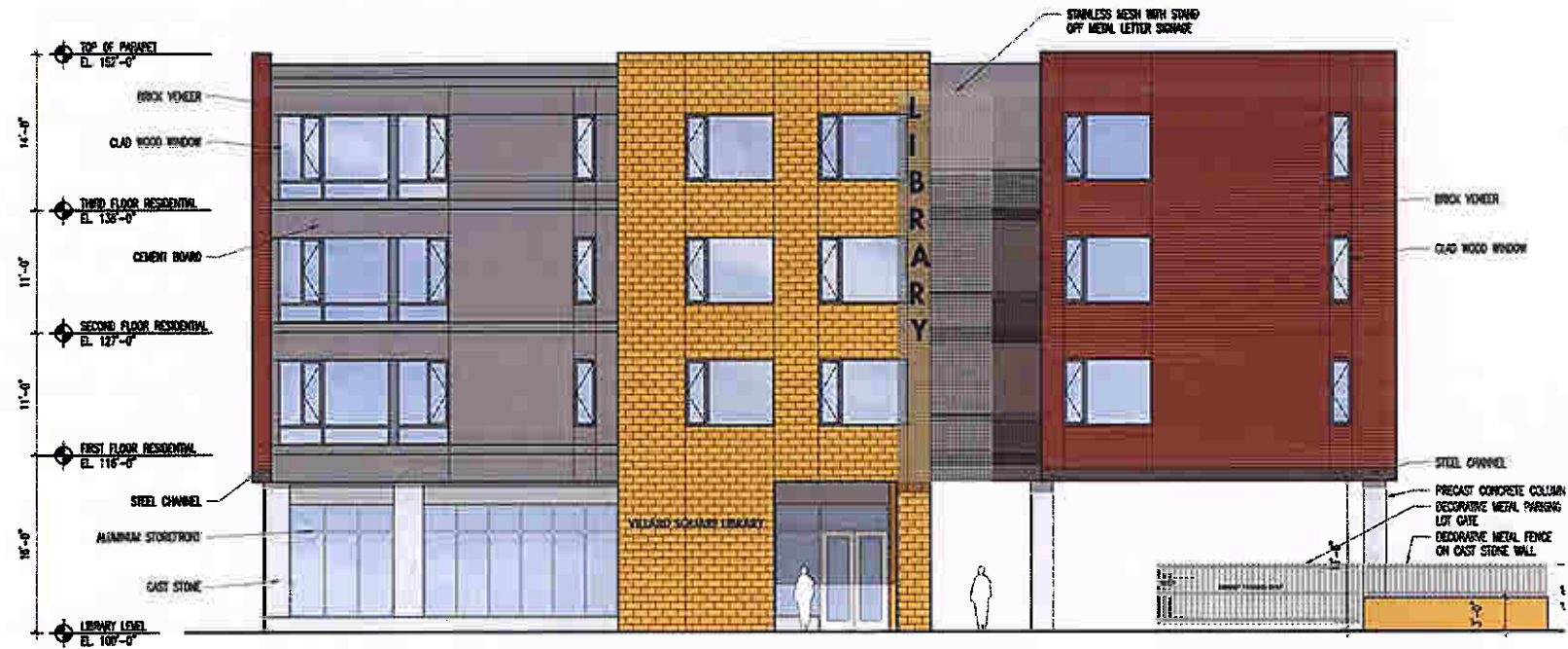
NORTH 35TH STREET ELEVATION SCALE: 1/8"=1'-0"
