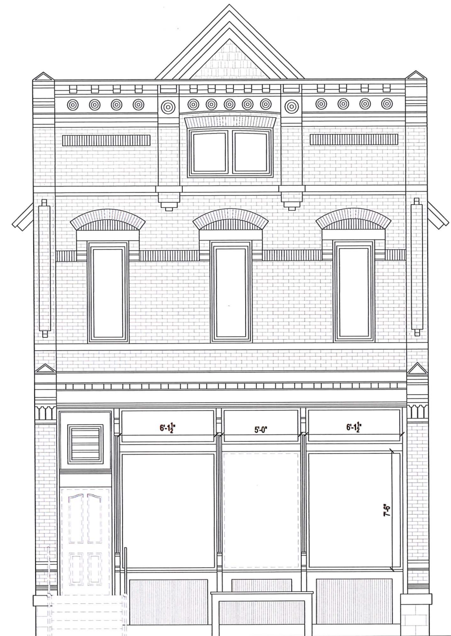
EXISTING SOUTH ELEVATION 3/8" = 1'-0" 2
