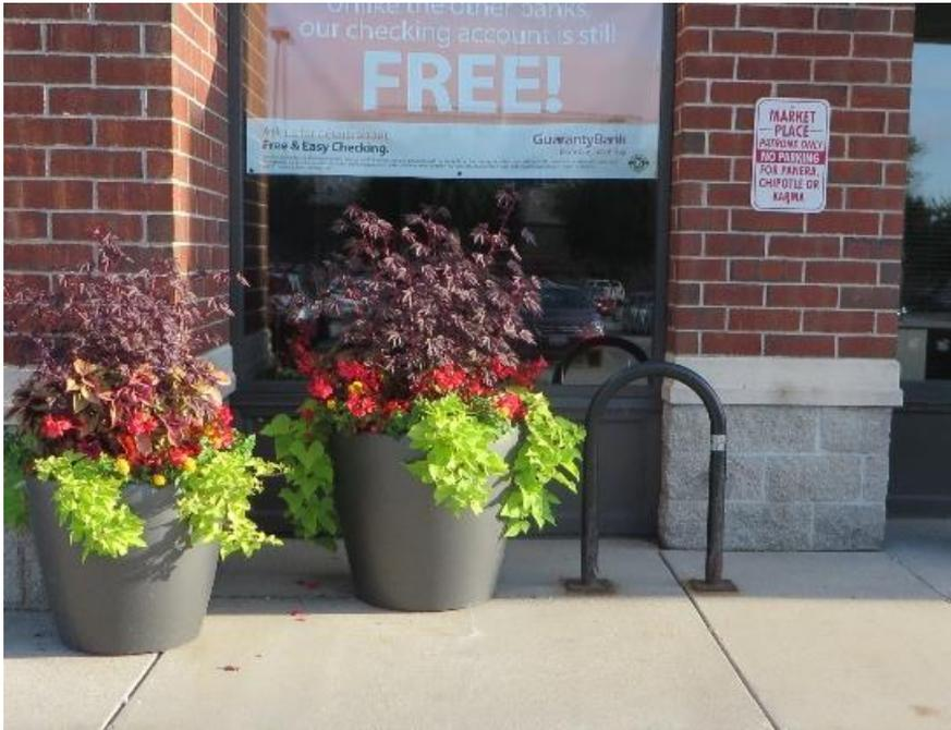
While an acceptable U-Rack, it is mounted too close to immobile planter to allow bike to positioned next to it.
