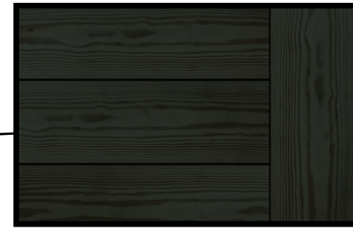
Decking and Stair Material: Treated wood decking, treads and cedar risers, all finished wood will be smooth and free of knots and have no visible injection marks. Paint with opaque stain to match existing building.
