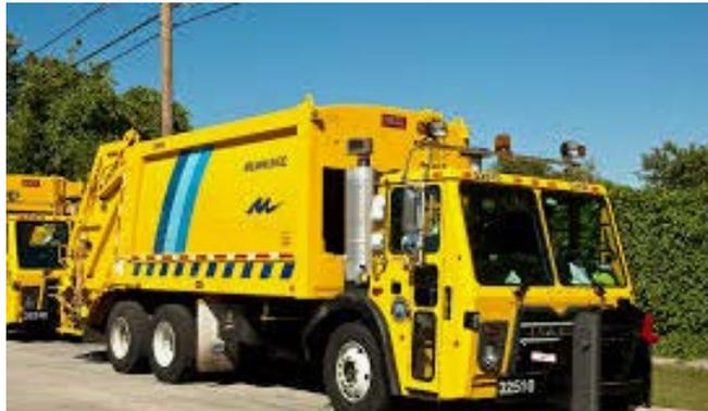
To cover the cost of purchasing CNG packers, the division has used Congestion Mitigation and Air Quality (CMAQ) grant funding. Under Wis. Stat. SPS 340.71, CNG systems must be operated and maintained as defined by code National Fire Protection (NFPA) 52, which requires that CNG cylinders must be inspected every three years or 36,000 miles, whichever comes first, or after any accident or fire. The scope of the review included all DPW CNG vehicles and equipment.
