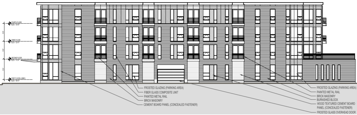
BUILDING 1 WEST ELEVATION SCALE: 1/8"=1'-0"
