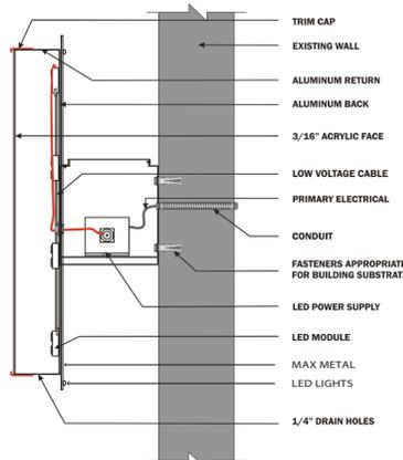
Standard Face Lit - LED Illuminated w/ Raceway
