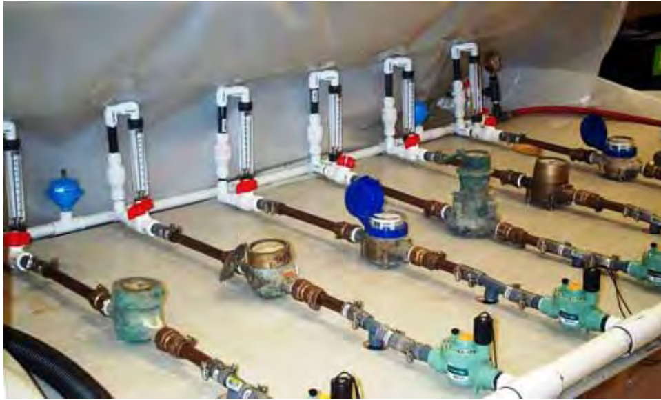
Figure C.35 Water meter test rig. Meters are numbered from left to right, with Meter 1 being the leftmost one and Meter 6 the rightmost.
