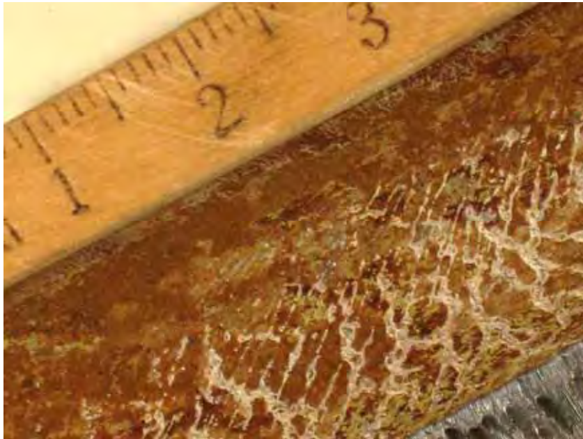
Figure F.38 Photograph of the Surface of Scale from Pipe PP03 (Site D1)
