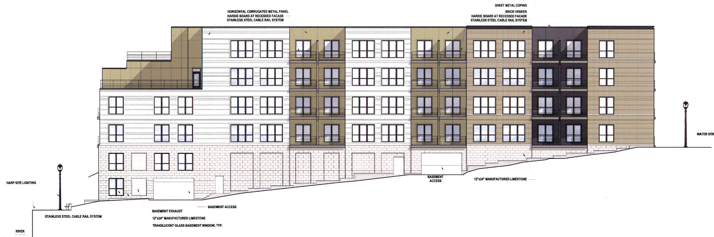
F1 BUILDING 2 - SOUTH ELEVATION SCALE: 1/8" = 1'-0"
